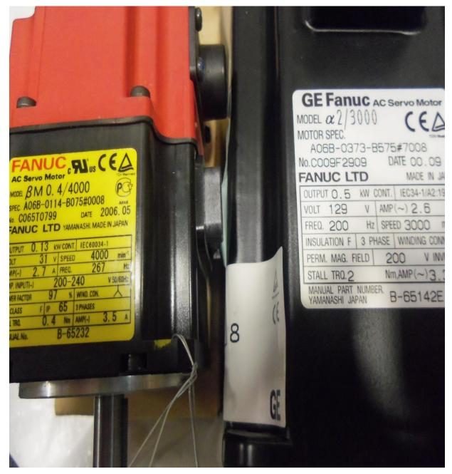
If the end of the motor shaft is not visible, check the tag on the motor to see if it is a yellow FANUC tag or a silver GE FANUC tag.
