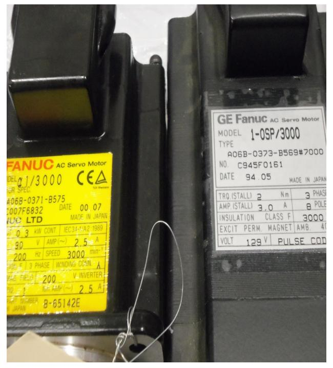
The above tags are **both** for a motor with a **slick shaft**. GE FANUC uses the designation #7000 for a slick shaft. FANUC **does not** use a # suffix for a slick shaft.
