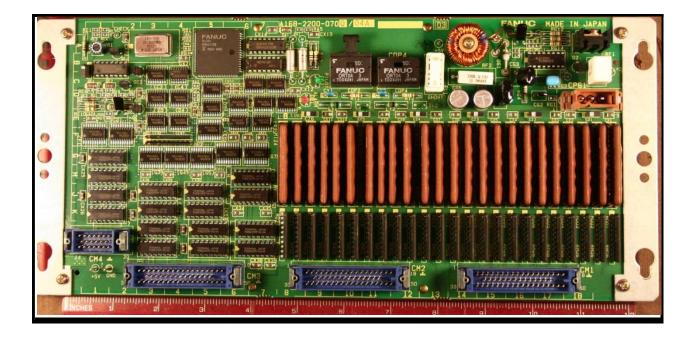
The VR1 pot in the upper left hand corner of this picture may have to be adjusted if the outputs are not working. The VR1 pot sets the firing level of the outputs. The firing level will vary from machine to machine. If you are having a problem with the outputs, then adjust VR1.
