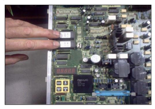
Failure to move the software from the old drive to the new drive will cause the display on the drive to be blank.
