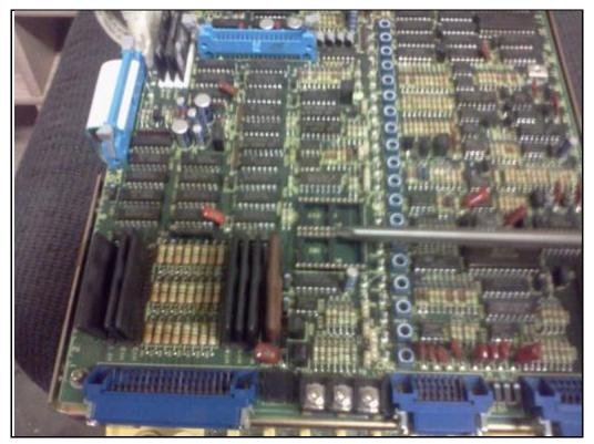
The DAC chip is an option chip. If the DAC chip is present on the old spindle PCB, it must be moved to the new spindle PCB and put into the same socket that was used on the old spindle PCB. Failure to move this chip can cause the spindle to rotate very slowly in automatic operation.
