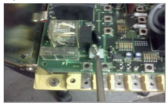
3. Move software chip from the old spindle PCB to the new spindle PCB.
